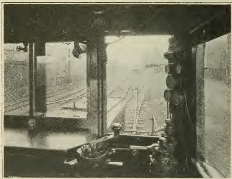
View showing visibility from operator's station on 60-ton Diesel electric locomotive.
